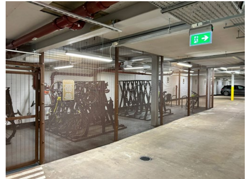
Cycle amenity at car park level with combination of semi-vertical cycle racks and sheffield stands - colour scheme matches interior scheme
